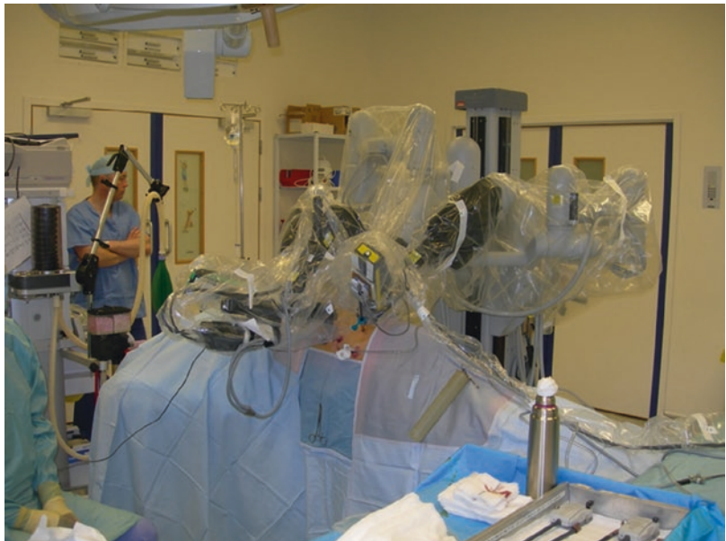
Fig. 5.1 Theatre set-up for a left pyeloplasty: note the position of patient, robotic arms, and anaesthetist. Reproduced with permission from Cundy et al. [2]
