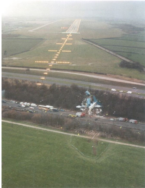
Fig. 4 The broken 737 lies on the western embankment of the M1 motorway. Note how the tail section jack-knifed up the embankment
