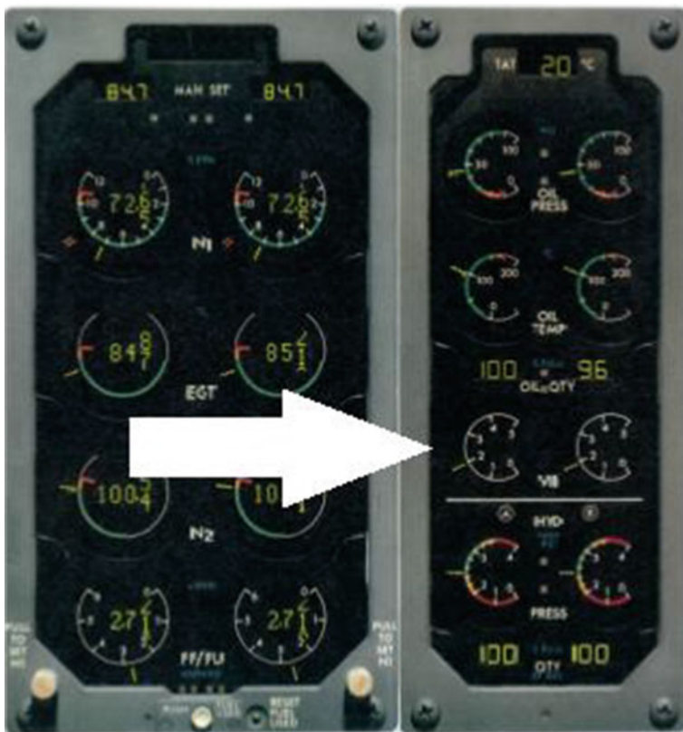
Fig. 3 The 737-400's primary and secondary engine displays. The engine vibration indicators are arrowed
