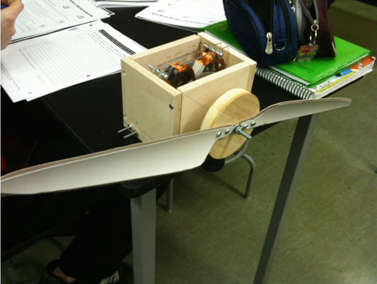
Fig. 1 A wooden windmill capable of producing up to 40 V
