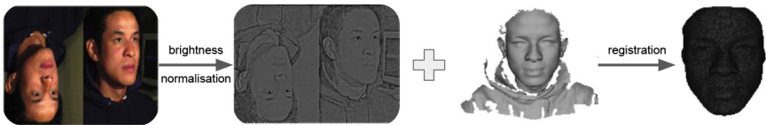
Fig. 5. Albedo 3DMM construction. Left to right: RGB and preprocessed texture map, shape, and registered face.
