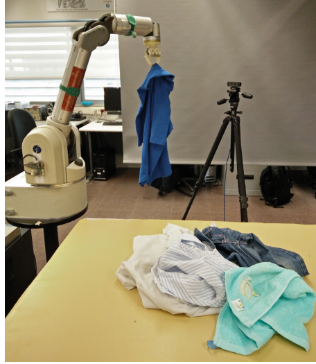
Fig. 1. Setup, including the robot manipulator, the Senz3D ToF camera, and the table where garments are lying.
