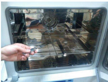
Fig. 14.5 Thermal cycling (heat cycle)
