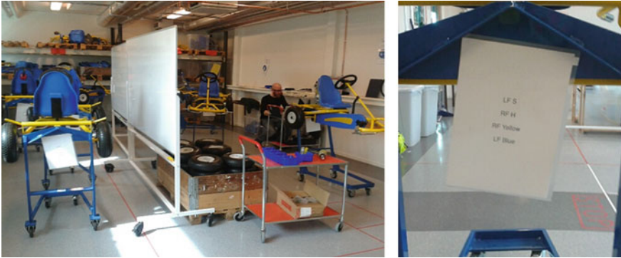
Fig. 2 The simulated assembly line to the left (a), and a closer look of a delivery note to the right (b)
