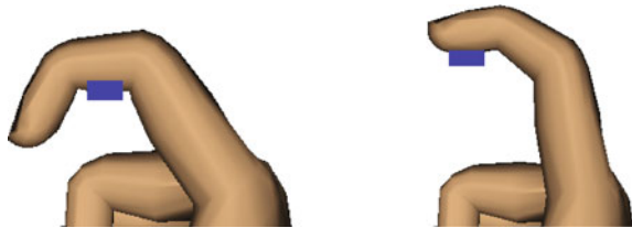
Fig. 3 Visualization of different trigger positions ( left side wrong trigger position, right side correct trigger position )
