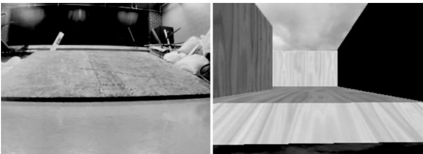
Fig. 1 Drive camera views from a Jaguar V4 UGV ( left ), and from the simulated Jaguar V4 platform in the Automated Navigation Virtual Environment Laboratory (ANVEL) simulation environment ( right )
