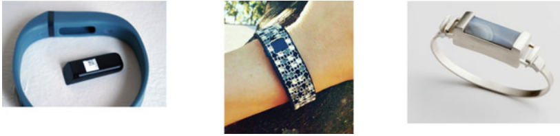
Fig. 2 A Fitbit flex with its tracker taken out and its accessory bands [19]
