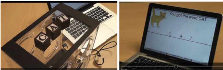
Fig. 3 On the left , manipulating augmented blocks on top of the surface. On the right the feedback displayed on the screen
