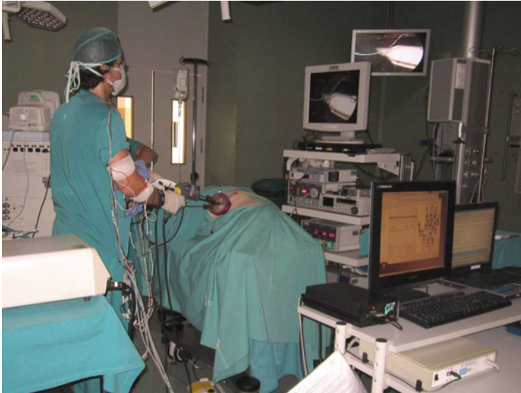
Fig. 3 Setup for the study with the animal model. The surgeon is using the robotic instrument with the needle holder end-effector during the surgical procedure. Surface electromyography is used to record the surgeon's muscular activity
