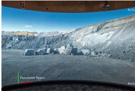
Fig. 1 Photo depicting the wrap point of the stimulus display. As shown on the image, the panorama coordinate space begins at the lower left of the panorama, with the x ( horizontal ) and y ( vertical ) axes running from (0,0) at the bottom left to (1,1) at the top right. Also shown is the buffer region above and below the image, which exists to ensure the panoramic image is uniformly level on the top and bottom, despite any small variations in screen height and projection region
