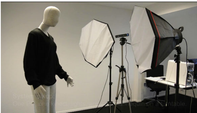
Fig. 2 The 3D cloth scanning setup using a mannequin doll and a Microsoft Kinect sensor
