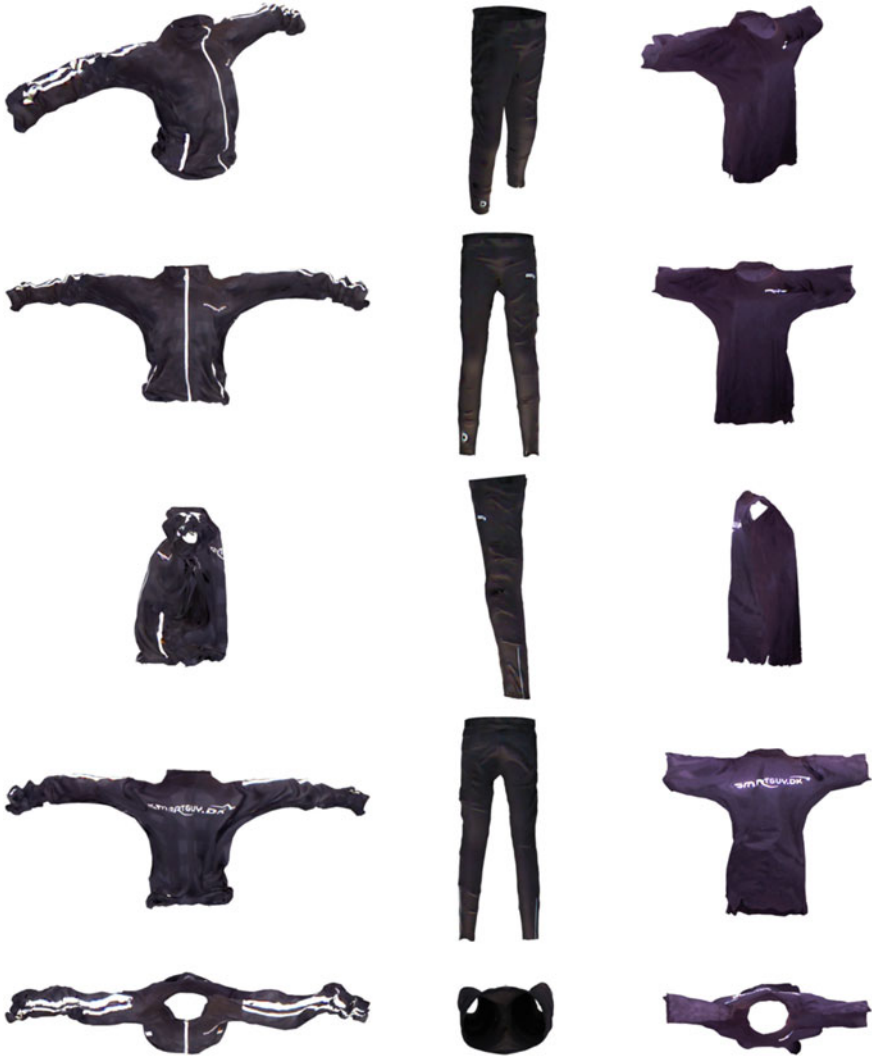
Fig. 7 Experimental results of scanning three different kinds of clothes (a shirt, a pair of pants and a T-shirt) displayed from multiple viewpoints
