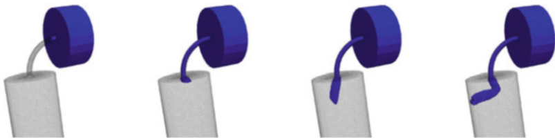
Fig. 21.32 Die swell of a visco-elastic fluid for a die with a 90 degrees bend. Snapshots of the solution at times t = 0, 0.4, 0.8, and 1.2 s (left to right).
