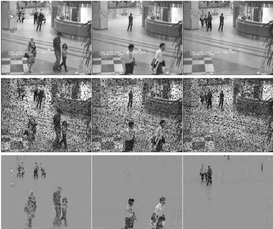
Fig. 6.4 The 10th, 100th, and 200th frames of the original surveillance video (first row), the corrupted video (second row), and the sparse video recovered from SC-PRSM-PR (third row).
