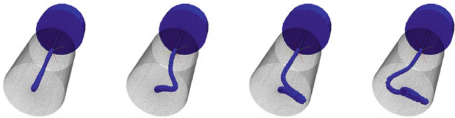
Fig. 21.16 Die swell with extrusion of a Newtonian fluid, with no-slip boundary conditions in the die ( \mu = 10 \text{ kg}(\text{ms})^{-1} ). Snapshots of the buckling of the jet at times t = 1.0, 1.2, 1.4, and 1.6 \text{ s} (left to right).
