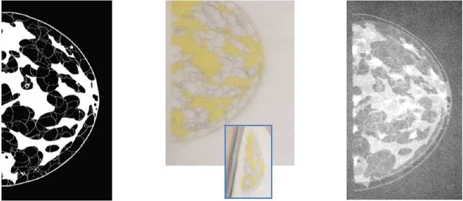
Fig. 1. Fabrication of physical phantom. The phantom was (a) designed as a virtual model, (b) realized through printing and (c) x-rayed on a mammographic system.
