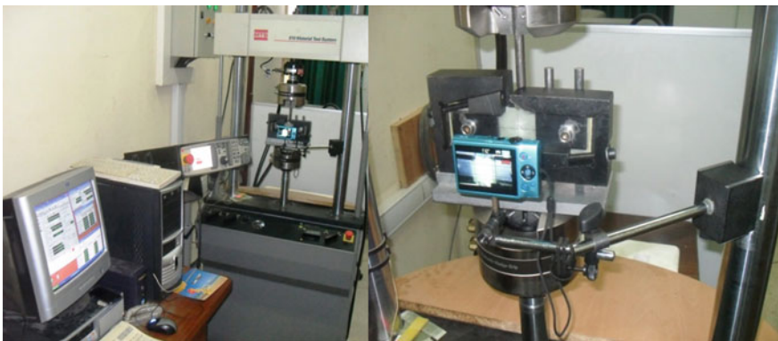
Fig. 4 Iosipescu device mounted on a MTS 810 machine
