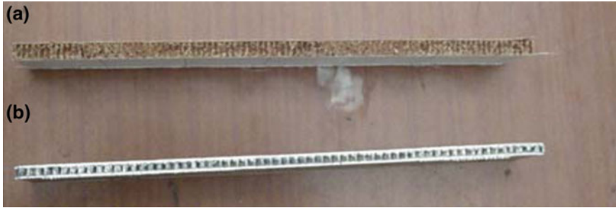
Fig. 1 Honeycomb sandwich beams with a Nomex and b Aluminum alloy cores
