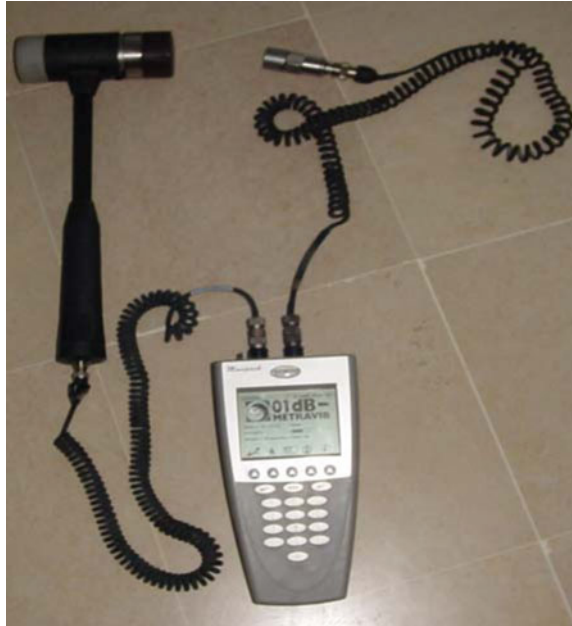
Fig. 2 Equipment: impact hammer, sensor and spectrum analyzer
