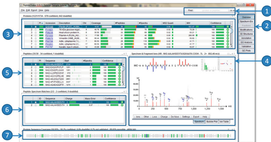
Fig. 11.1 PeptideShaker overview tab: (1) the search box allows for targeted investigation of proteins and peptides; (2) select other tabs for additional analysis and quality control; (3) the protein table displays details on the proteins identified in the dataset; (4) the peptide table lists details on the peptides used to identify the
