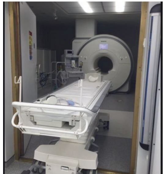
Fig. 22.1 The iMRI dual-room suite with the docking trolley in front and an MRI-compatible ventilator by the side of the stationary magnet (Picture courtesy of Centre of Image Guided and Minimally Invasive Therapy – CIGMIT, University Malaya Medical Centre)
