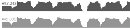
Fig. 6. Timeline view of a bandwidth utilization on MIC with original AoS memory layout when running core engine of the NEURON simulator. The first trace is a read bandwidth, whereas the second trace is the write bandwidth (in GB/s).
