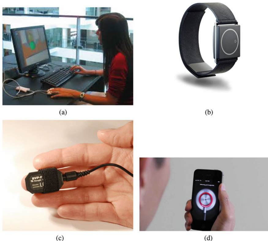
Fig. 7.1 The key physiological signal sensors and devices discussed in this chapter. (a) The IOM device used during the data collection experiment reported in [109]. (b) Empatica's Embrace wristband. (c) The blood volume pulse sensor of the ProComp Infiniti device. (d) The Cardio application for smartphones
