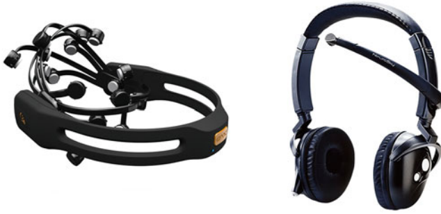
Fig. 6.1 BCI devices. On the left – Emotiv Epoch; image available at http://emotiv.com , On the right – Neurosky Mindset; image available at http://neurosky.com . Epoch is a trademark of Emotiv, Mindset is a trademark of Neurosky (Images used with permission)
