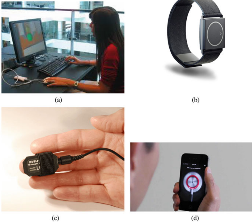
Fig. 7.1 The key physiological signal sensors and devices discussed in this chapter. (a) The IOM device used during the data collection experiment reported in [109]. (b) Empatica's Embrace wristband. (c) The blood volume pulse sensor of the ProComp Infiniti device. (d) The Cardio application for smartphones
