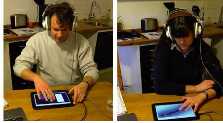
Fig. 1. Experiment setting: two blind participants equipped with a headphone trying to identify a box plot (left) and a mathematical function plot (right) by moving their finger on the tablet surface
