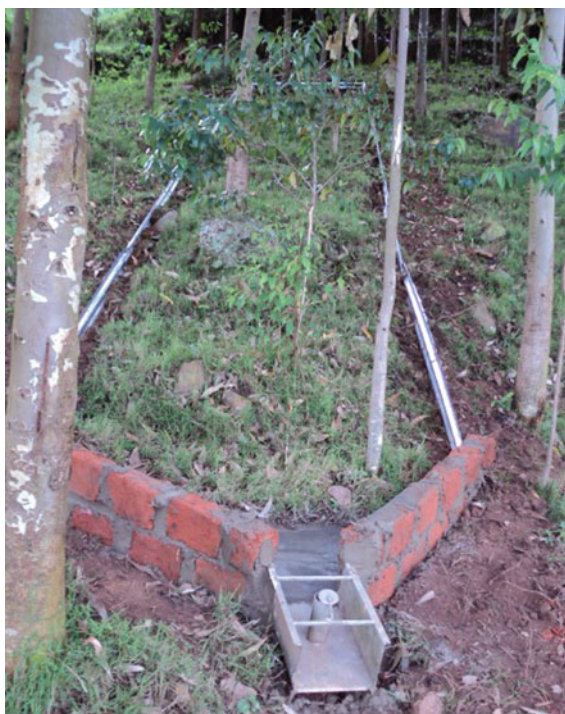
Fig. 10.2 Erosion plot constructed in a woodlot in L. Bunyonyi catchment
