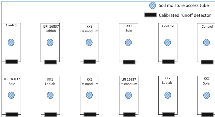
Fig. 22.2 Experimental set up of forage-grass and forage-legume interactions showing soil moisture access tubes and runoff soil trap detectors with each plot measuring 10 m × 5 m
