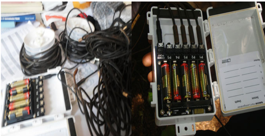
Plate 29.1 Temperature sensors and data logger
