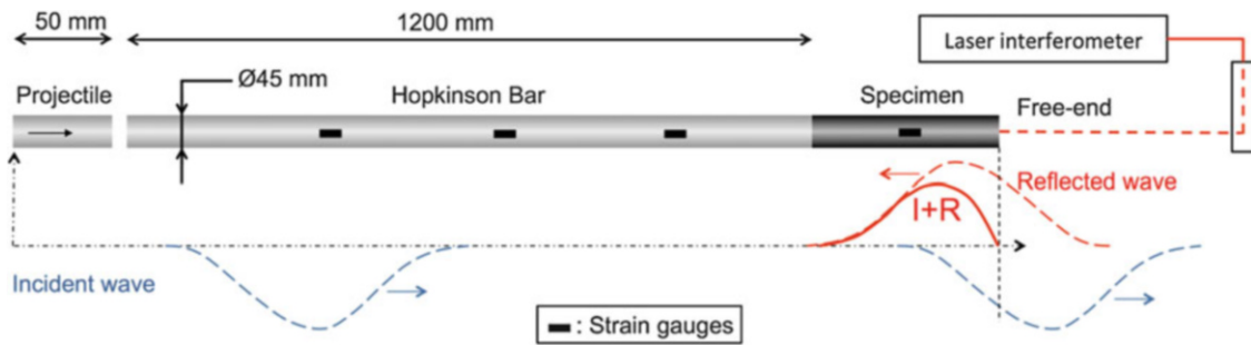
Fig. 17.1 Experimental device for spalling tests
