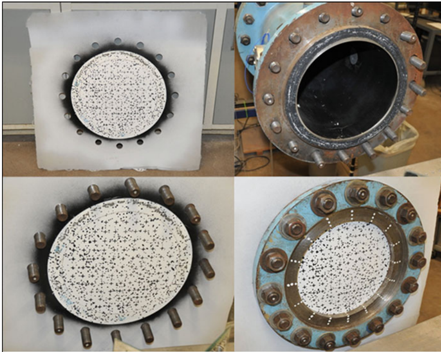
Fig. 13.5 Clockwise from top left: composite plate drilled for bolt-through mounting, gasket in place on shock tube working section flange, plate placed on mounting bolts, retaining ring bolted in place
