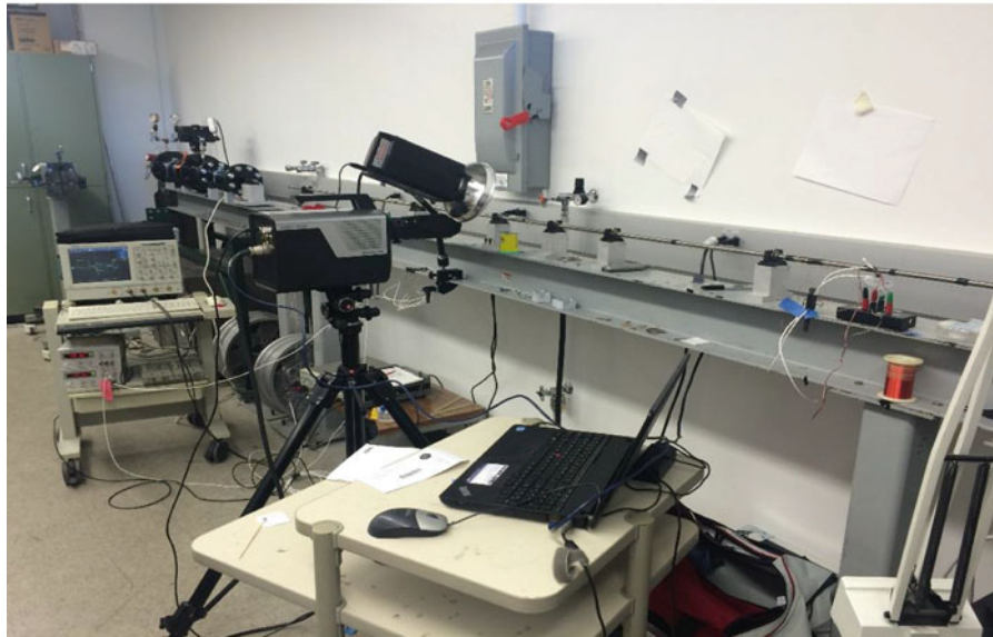
Fig. 5.8 Split Hopkinson compression bar
