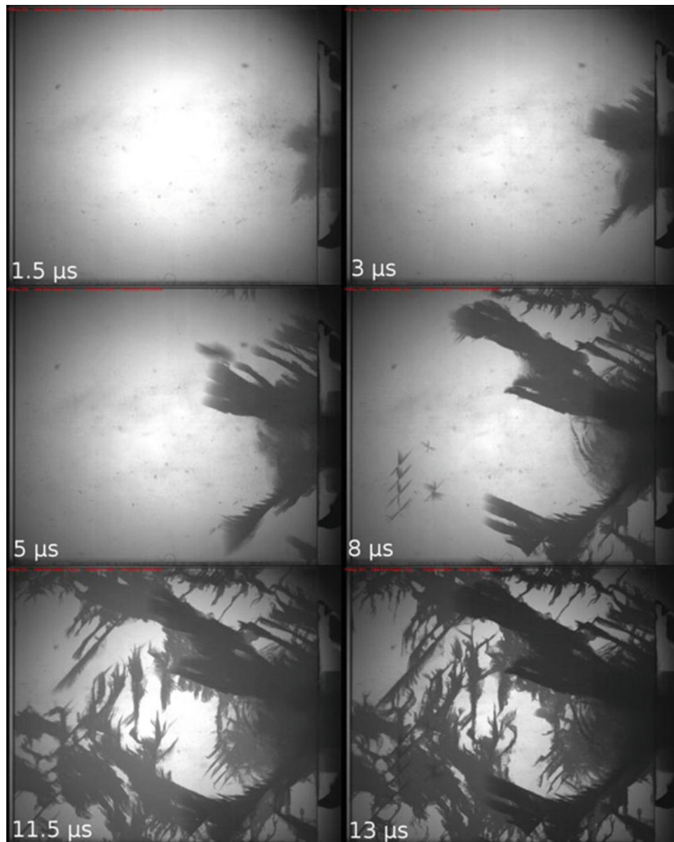
Fig. 23.5 S4 edge-on impact test performed at 227 m/s. Impact direction orthogonal to the C axis
