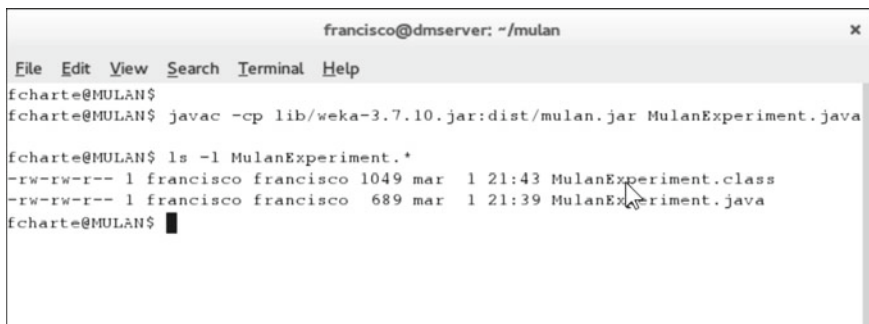
Fig. 9.31 To compile a MULAN program, the paths to the mulan.jar and weka.jar files have to be provided
