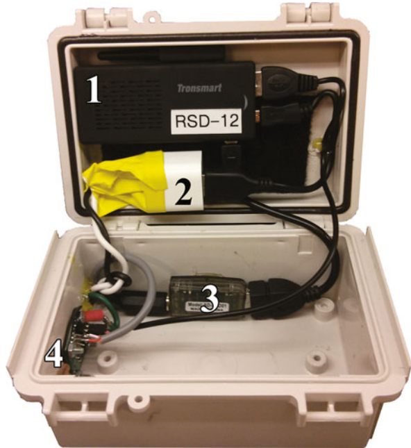
Fig. 3 Fixed-RSD (1 mini PC, 2 power supply, 3 audio interface, 4 MEMS microphone board)
