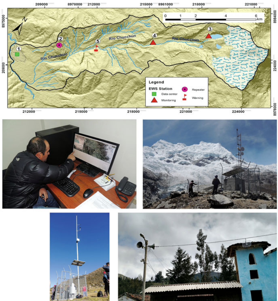
Fig. 12 Location map of the EWS monitoring network (above). Below, left to right: Data Center (1), Lake 513 station (3), Shonquillpampa Station (4), Pariacaca Station (5). Glaciares Project Photographic Archives
