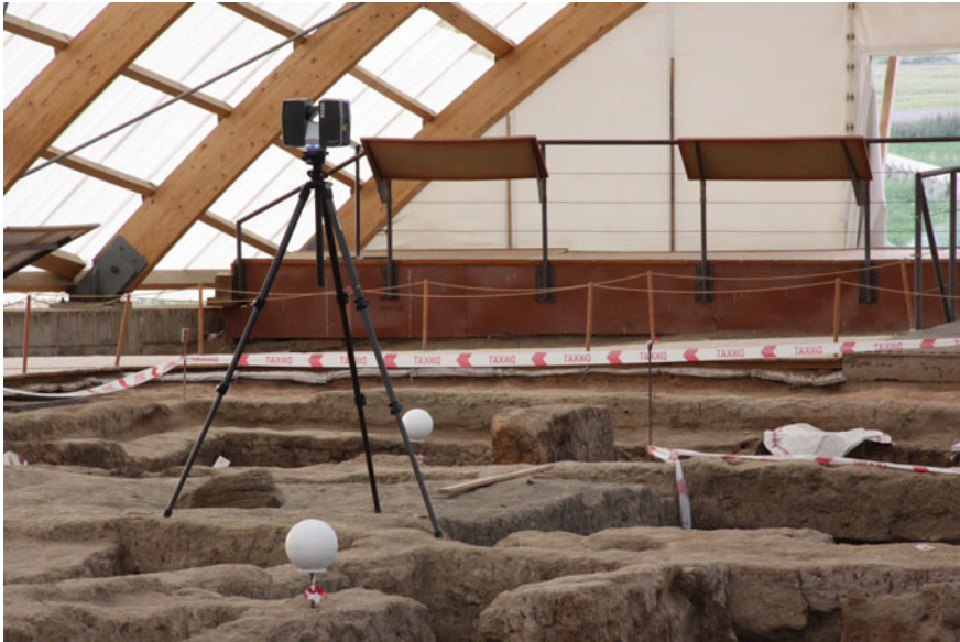
Fig. 8 FARO Focus 3D S120 scanning Neolithic buildings in the North Area of Çatalhöyük's East Mound
