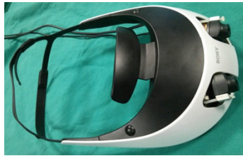
Fig. 1. Modified HMD display. The two external cameras can be moved to adjust eye convergence and field of view.
