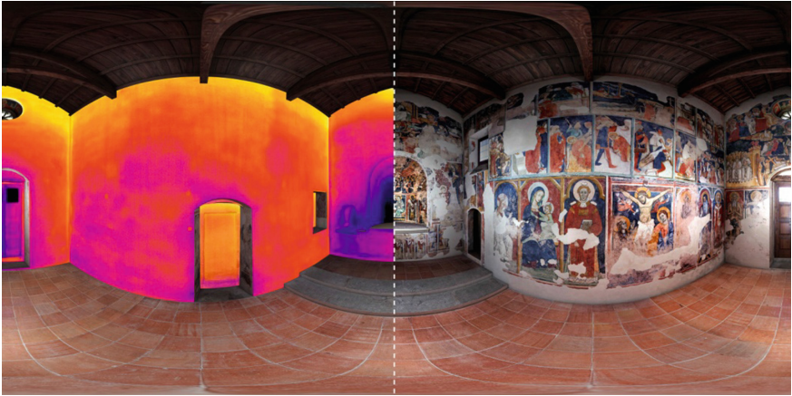
Fig. 9. Spherical panoramas with IR analysis (left) perfectly matched over visible colors. (Color figure online)
