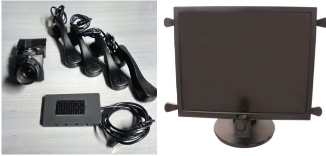
Fig. 2. The necessary hardware components (left): camera, infrared illuminators, and power distribution plug for the illuminators. A sample installation of EyeAssist (right), with details on the camera and light positioning
