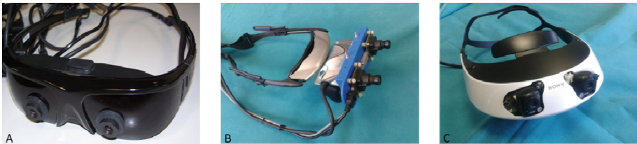
Fig. 2. Stereoscopic HMDs on which the software framework was tested. (A) Commercial video see-through AR visor by Vuzix (Vuzix WRAP 920AR). (B) First custom-made embodiment of stereoscopic HMD based on a commercial 3D visor by eMagin (eMagin Z800). (C) Second custom-made embodiment of stereoscopic HMD based on a commercial 3D visor by Sony (Sony HMZ-T2).
