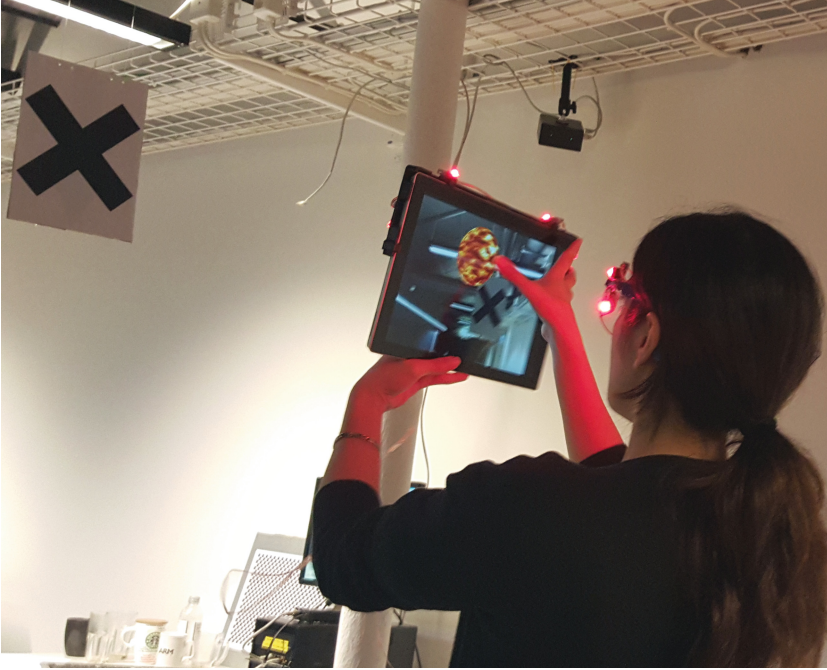
Fig. 3. The find-and-select test: Finding and selecting thirty virtual Spheres in one of the four pre-defined positions in 3D space in relation to the physical signs placed in the test environment.
