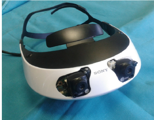
Fig. 1. Our custom-made stereoscopic video see-through HMD based on a commercial 3D visor by Sony (Sony HMZ-T2).
