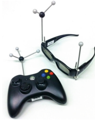
Fig. 2. The 3D goggle and gamepad controller with retro-reflective markers
