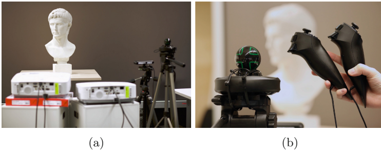
Fig. 3. (a) An exemplary setup of our system with two projectors, a depth camera for tracking and our Augustus bust as the target object. (b) The Razer Hydra we use for painting.
