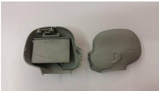
Fig. 5. The fetal head: on the left there are the grooves created to contain the electronic components, on the right a suture is visible
