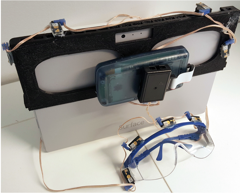
Fig. 2. The system prototype: Back side of the tablet computer with the 3D printed frame attached to it. The frame holds the illuminative markers and the LED unit driver that also is the power source for the LED markers. The safety goggles attached with illuminative markers that also is connected to the unit driver.
