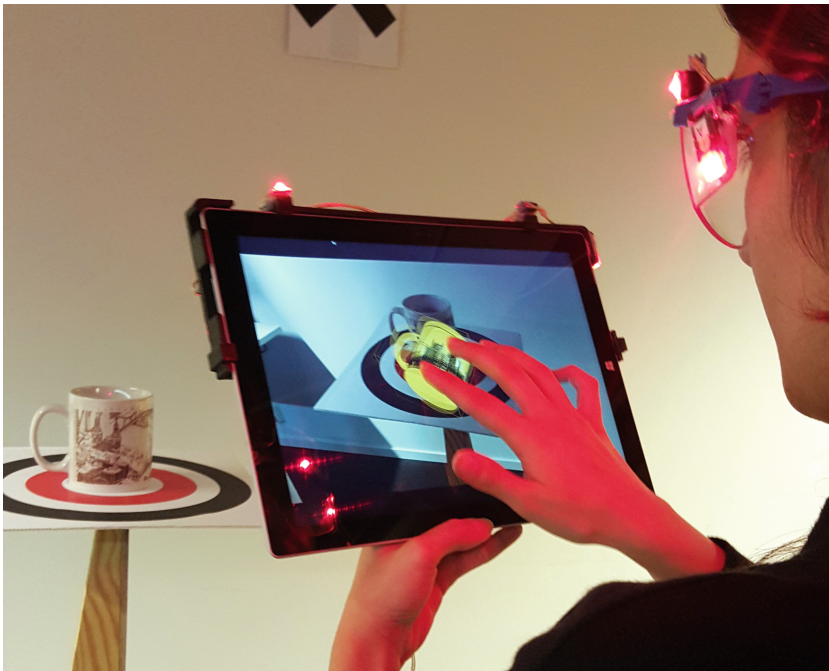
Fig. 6. Multi-Touch pose manipulation Test: Moving the virtual model of a coffee mug from a start point to an end point and aligning its orientation with a real coffee mug placed at the end point. The multi-touch interaction is used for the pose manipulation of the virtual object.
