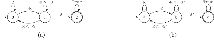
Fig. 7. Example: (a) safety specification \varphi^s(R, S) and (b) correctness monitor \mathcal{Q}(R, S') .
