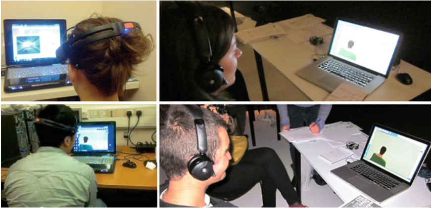
Fig. 12.16 Brain-computer interaction using the NeuroSky MindSet ( left ), brain-computer interaction using the Emotive device ( right )
