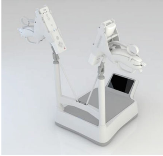
Fig. 6.6 The laparoscopic controller as a custom input device: two regular Wiimote game controllers are integrated in the device (Source CuttingEdge 2015)
