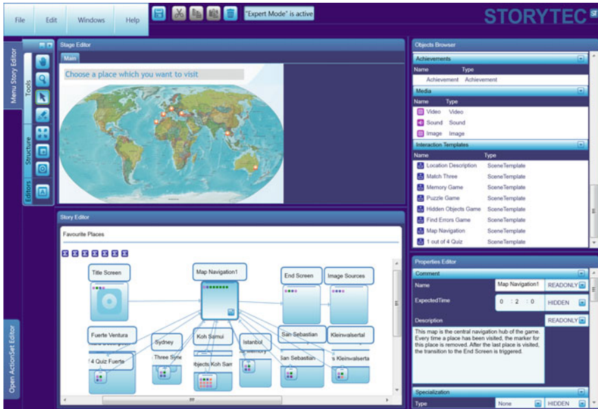
Fig. 4.7 The user interface of StoryTec. The Story Editor in the lower left part visualizes the overall game model, while the Stage Editor in the upper left part allows authors to change parameters of one scene interactively
