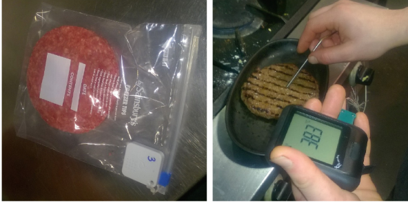
Fig. 4. Wireless tag attached to a pack containing a single raw burger (left). Wireless meat probe used to measure the core temperature of a burger during cooking (right).
