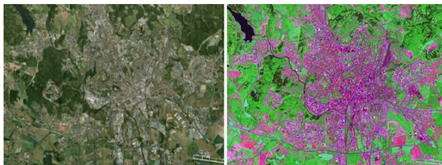
Fig. 1 Cutouts from LANDSAT images, left true-colour satellite image, right false-colour image (Source TopGIS)
