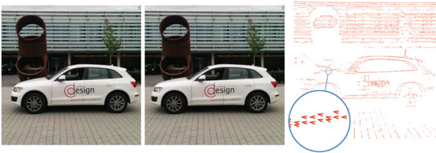
Fig. 5 Optical flow of an image sequence showing a driving car
