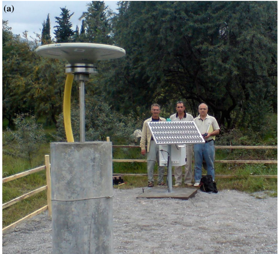
Fig. 6.15 a GPS continuously recording station located in Sheki, Azerbaijan. In the background, the project participants are shown (from left to right ): Prof. R. Reilinger, Dr. S. Mammadov, and Prof. F. Kadirov b GPS survey site in the Greater Caucasus. The antenna is precisely located above the mark that is cemented into the bedrock
