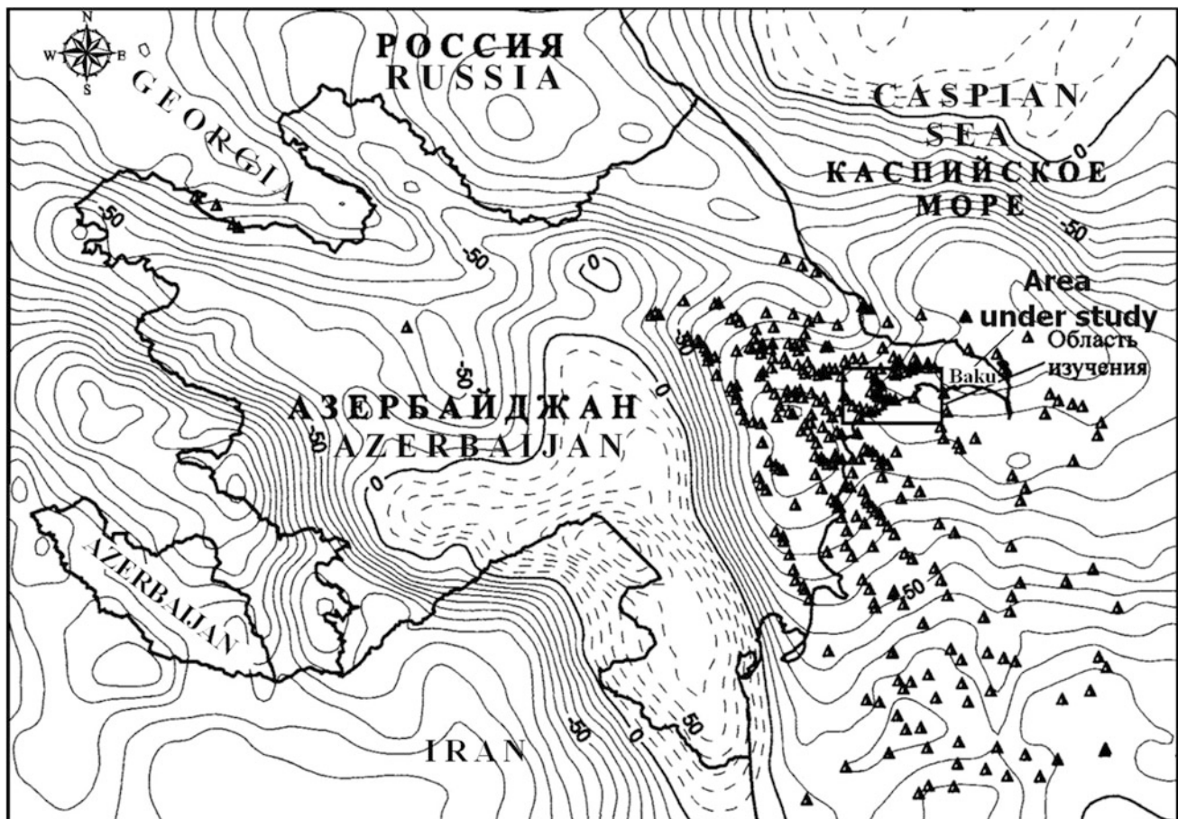
Fig. 9.5 Distribution of mud volcanoes (black triangles) in Azerbaijan and Bouguer gravity data (Kadirov and Mukhtarov 2004). Isoanomals (in milligals): solid lines denote negative values, and dashed lines denote positive values
