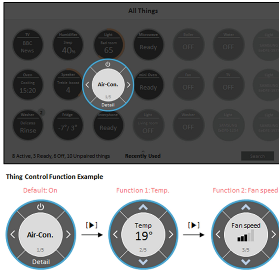
Fig. 5. (a) Things control in All Things of ETG, (b) Example of Things control function
