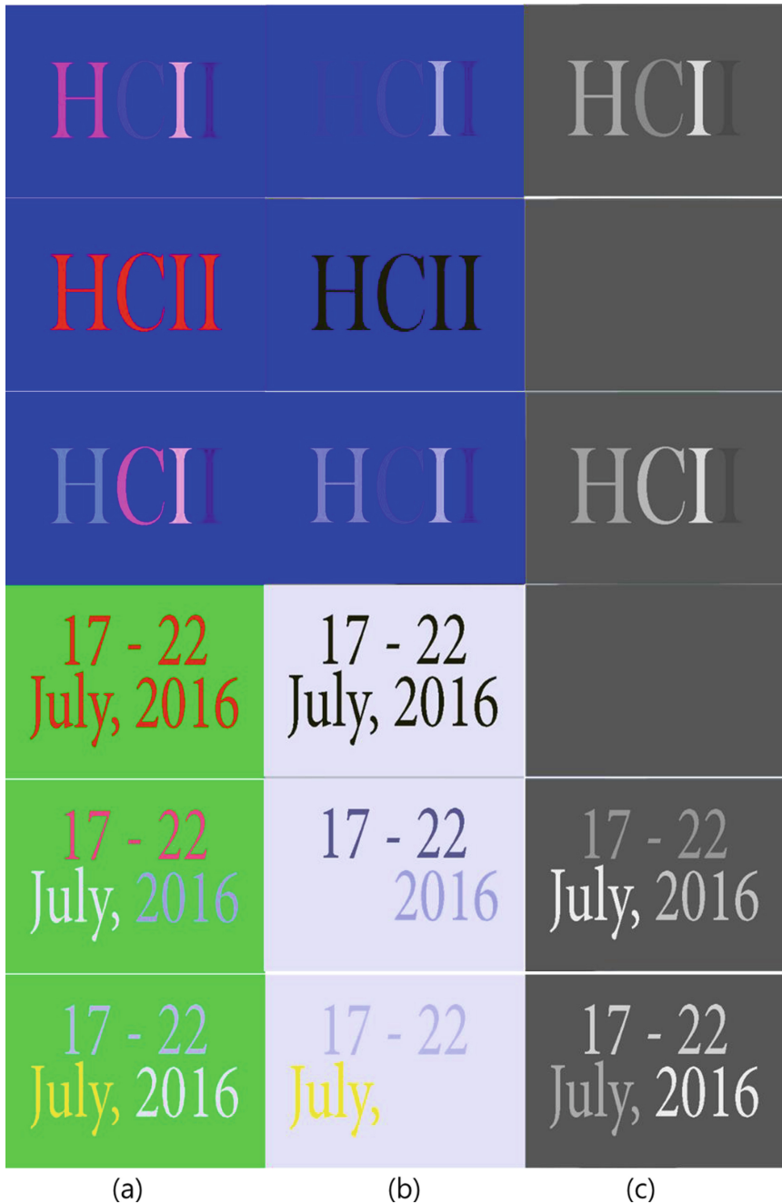
Fig. 4. Simulation results of various graphic designs (a) original graphic designs (b) simulated models for a person with protanopia (c) simulated models for gray-level printing
