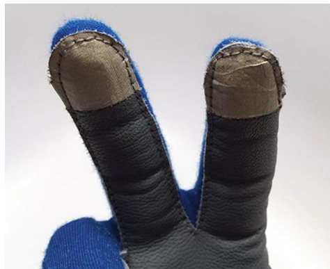
Fig. 4. Flying gloves used in the study, with conductive fabric on index and middle fingers
