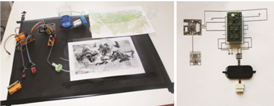
Fig. 6. Left: Current prototyping circuit. Right: Next iteration of portable micro-pumps for wearable applications.
