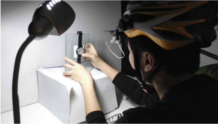
Fig. 3. The tester is conducting usability test experiment of Moto360 smart watch interface
