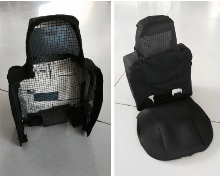
Fig. 8 The seat cover costume includes two arm outlets so that the concealed driver could steer the car using the bottom of the steering wheel
