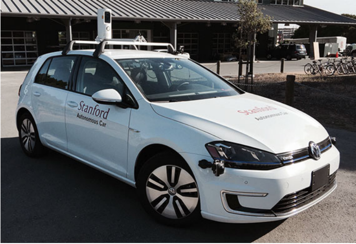
Fig. 7 The Ghost Driver car features autonomous vehicle props like a laser-based detector, radar units, interior and exterior cameras and decals on the hood and doors
