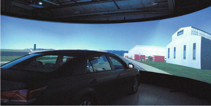
Fig. 1 The simulator used for experiments in autonomous vehicle driving and control. Participants sit in a fixed-base car surrounded by a 270° screen depicting the study environment
