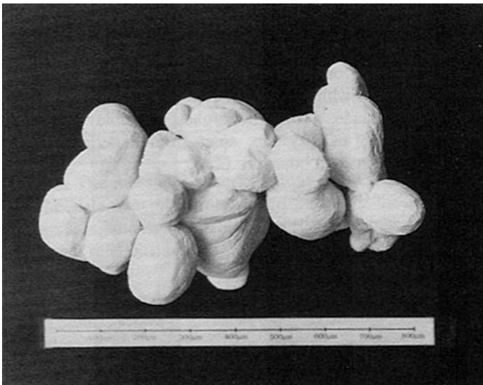
Fig. 4.33 3D reconstruction showing the interconnection of single agglomerate (reprinted with permission of The Minerals, Metals and Materials Society) [106]
