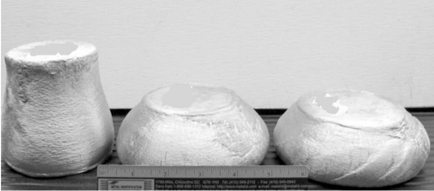
Fig. 5.8 As-deformed billets under 4.8 kPa applied pressure, cast at 695 °C, 630 °C, and 615 °C, from left to right , respectively [4]
