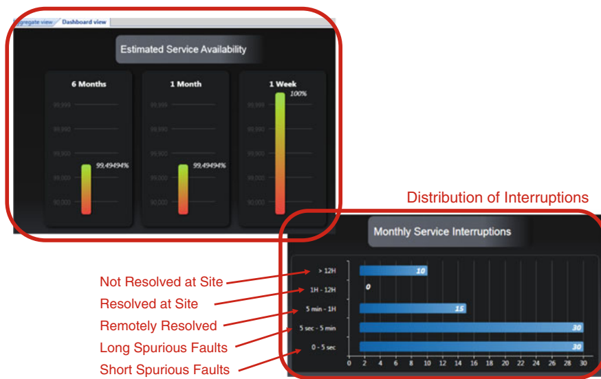
Fig. 18.1 Service availability and outage statistics as part of a Service Dashboard (Courtesy of GE Grid)
