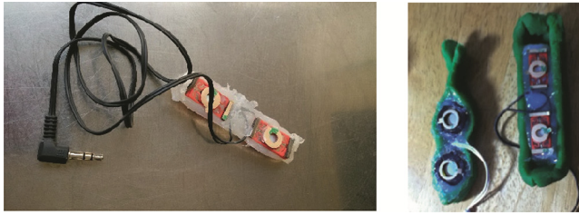
Fig. 3 a and b. Early prototyping showing transducer pair in silicone
