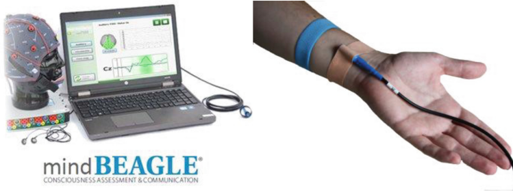
Fig. 1. The left panel shows the mindBEAGLE system. The right panel shows a close-up of the vibrotactile stimulators attached to the wrists. The right panel also shows the optional anti-static grounding straps. Usually, mindBEAGLE obtains adequate quality signals without any grounding strap, however in rare settings they can be used to reduce noise.
