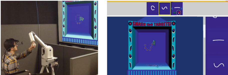
Fig. 2. Left – Patient, Game and Robotic Arm interaction, Right – Therapist's screen for online session adaptability that displays duplicate view of the patient's game-play (center), current exercise program (top) and available exercises (right).
