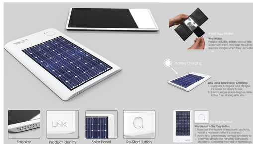
Fig. 8. Product design details of LINK and further explanation of key features.
