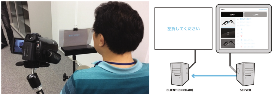
Fig. 1. Figures showing (a) view of system setup from behind where the opaque display mode is being used, and (b) network setup for server and client software and hardware.
