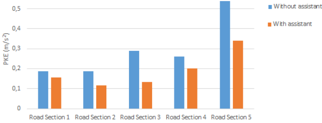
Fig. 4 Positive Kinetic Energy ( m/s^2 ) using the speed assistant
