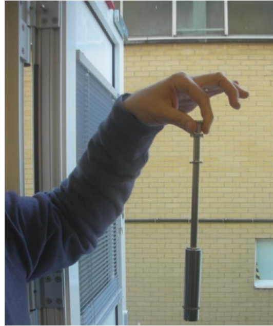
Fig. 2.4 Long-handled tool for handling stock vial
