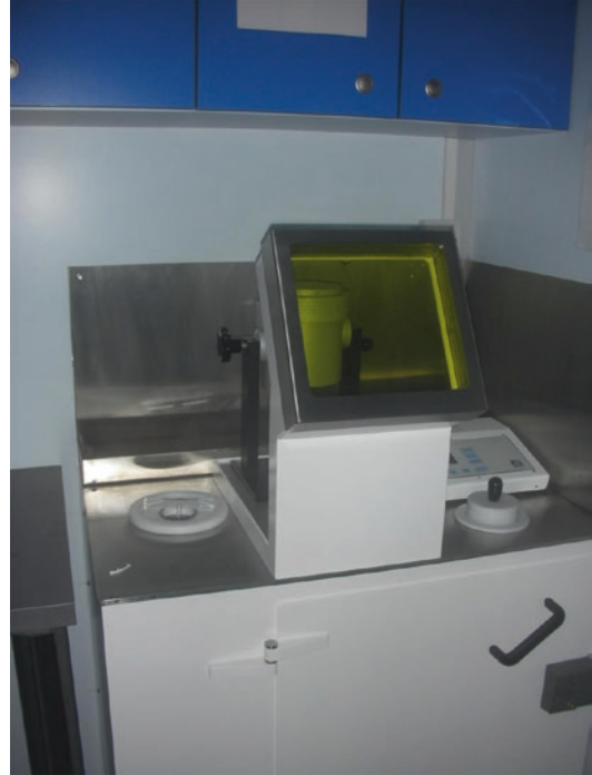
Fig. 2.6 Dispensing unit with bench top shield, sunken calibrator and waste route into shielded cupboard
