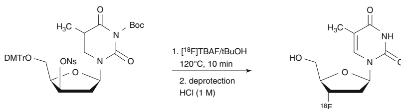
Fig. 4.4 Synthesis of ^{18}\text{F} -FLT by reaction in tert-butyl alcohol of the protected using ^{18}\text{F} TBAF as phase transfer catalyst
