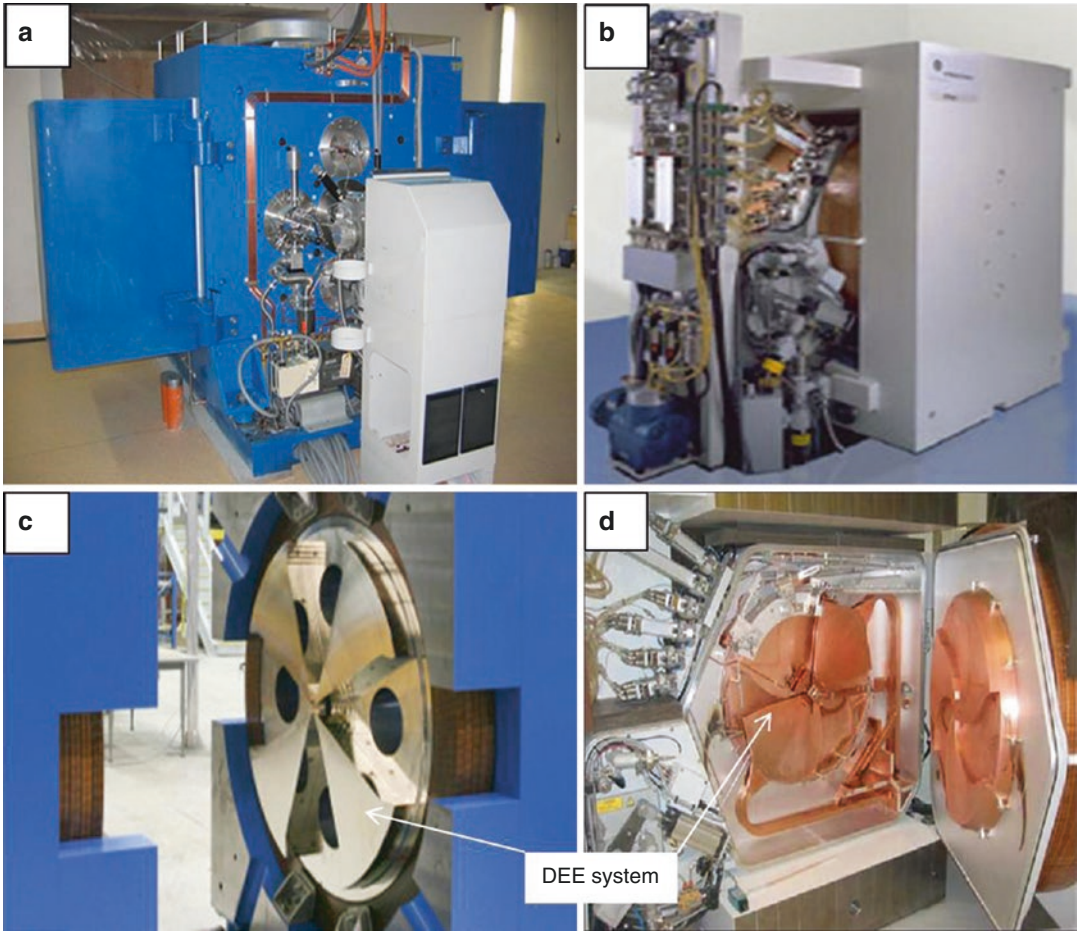
Fig. 1.8 Medical cyclotron for radiopharmaceuticals productions. (a) ACS cyclotron TR-24 (24 MeV) high current cyclotron for production of PET and SPECT radionu-
