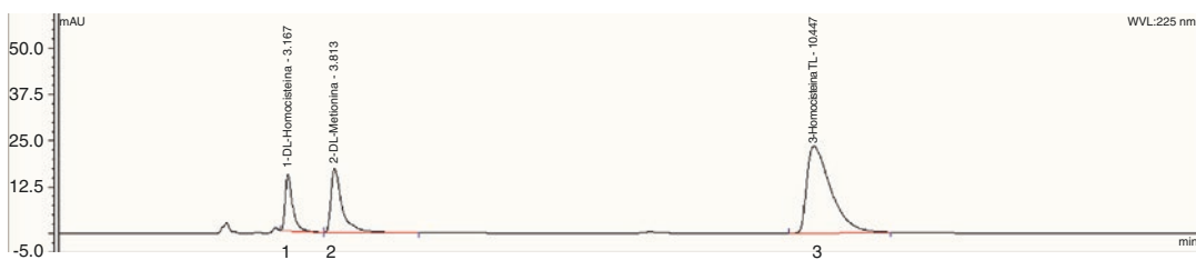
Fig. 5.4 HPLC chromatogram of standard solution for chemical purity of ^{11}\text{C} -methionine: 1: DL-homocysteine, 2: DL-methionine and 3: L-homocysteine thiolactone
