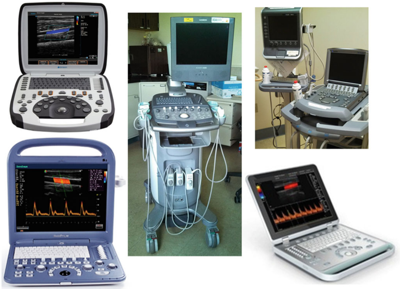
Fig. 22.1 Laptop-sized portable ultrasound units with high-quality imaging facilitate point-of-care applications. Clockwise from top left : Terason uSmart 3300, Siemens Acuson X300, Sonosite S Nerve and M-Turbo, Mindray HUC5-3D, and Chison Q5
