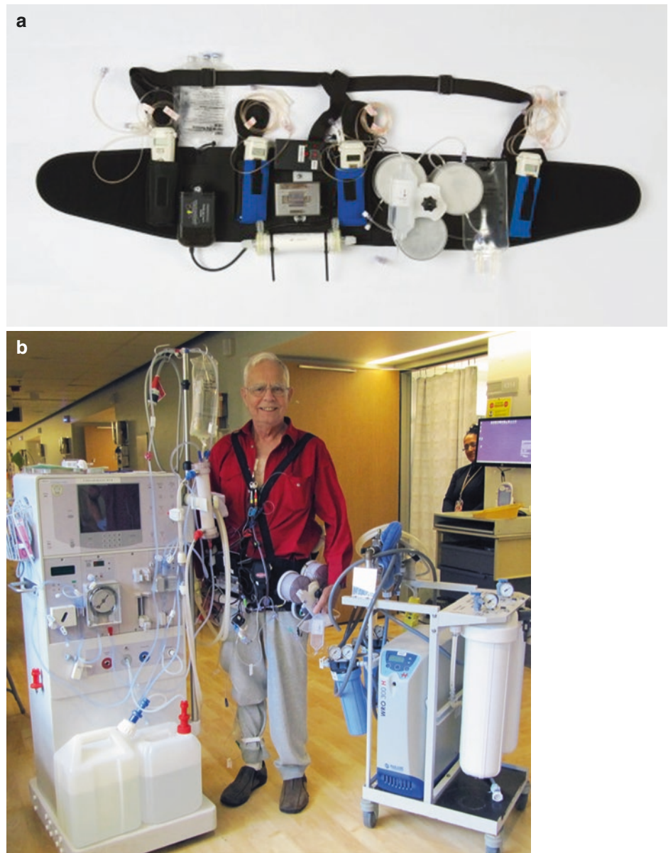
Fig. 42.2 (a) Belt-based wearable hemodialysis unit, the wearable artificial kidney (WAK) (Courtesy of Stephen Brashear for UW Medicine). (b) Chuck Lee was the first US patient to don the wearable artificial kidney in a clinical trial of the device, at UW Medical Center standing in contrast to two less-portable dialysis options (Courtesy of Sandy Lee for UW Medicine)
